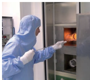
Annealing furnace in clean room environment
