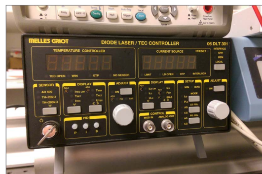
Driver de diode laser
